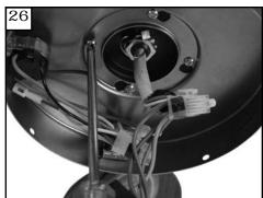
Install switch housing plate by twisting plate with key hole slots into place. Replace screw removed and tighten the 4 screws securely.
